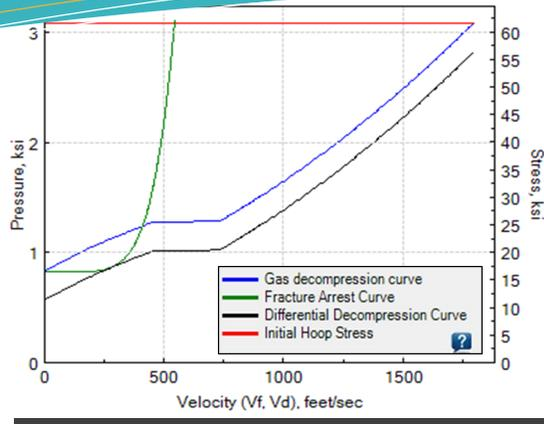
Emc<sup>2</sup>PDFA allows the user to predict unstable axial ductile fracture behavior in high energy pipelines to:
